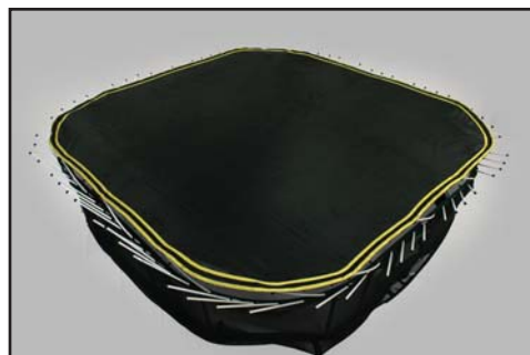
Figure 13-A: Every fifth rod attached to the mat
