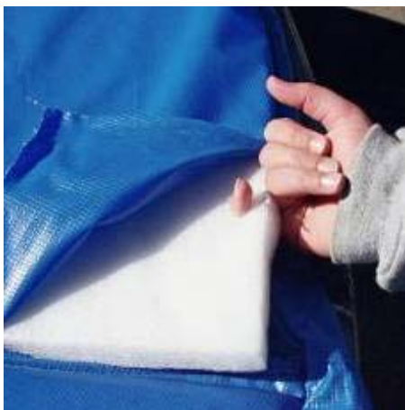
Figure 2: Korean trampoline – Failed AS 4989 impact test above a support leg
