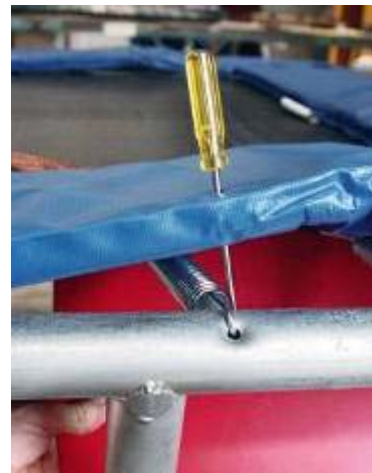
Figure 1: Chinese trampoline – Failed AS 4989 impact test above a support leg
