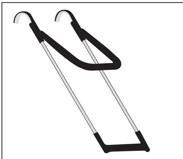
**Step 3:** Hook the FlexrStep™ over the frame below the enclosure door entrance.
