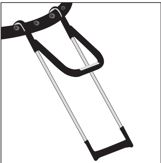
**Step 4:** When not in use, always ensure net is locked and remove FlexrStep™ to restrict access to the trampoline.
